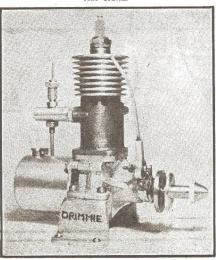
port,  $\frac{1}{4}$  h.p.; recommended propeller, 13" dia.,  $7\frac{1}{2}$ " pitch.
